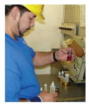
Glycol causes chilled-water system fouling and that means Hartford Steam Co. has to check system bacteria counts daily, regularly adjusting the amount of chemicals added - all of which increase chilled-water costs.
